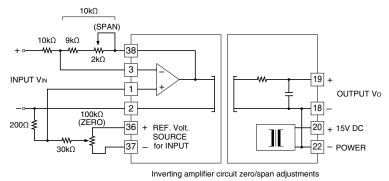
For an inverting amplification with external adjustments, when the combined resistance of the span adjustment and 9 k $\Omega$  is 10 k $\Omega$ , the gain is -(10 k $\Omega$ /R<sub>2</sub>) × VIN. With the span adjustment (2 k $\Omega$ ), the output is configurable. The zero is adjustable with a reference voltage source of ±16.5 V DC and the attenuation of 200  $\Omega$  and 30 k $\Omega$ .
