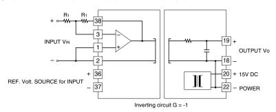
The output is inverted from the input. The gain is -1.
