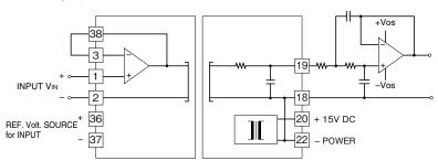
Circuit with low-pass filter installed on the output.
