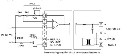
For a non-inverting amplification with external adjustments, when the combined resistance of the span adjustment and 9 k $\Omega$  is 10 k $\Omega$ , the gain is (1 + 10 k $\Omega$  / R<sub>2</sub>) × VIN. With the span adjustment (2 k $\Omega$ ), the output is configurable. The zero is adjustable with a reference voltage source of ±16.5 V DC and the attenuation of 200 $\Omega$  and 30k $\Omega$ .
