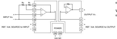
Non-inverting amplifier circuit G = 1 + R<sub>1</sub> / R<sub>2</sub>
