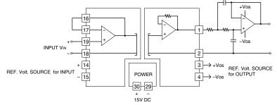
For a non-inverting amplification with external adjustments, when the combined resistance of the span adjustment and  $9k\Omega$  is  $10k\Omega$ , the gain is  $(1+10k\Omega$ /  $R_2)\times VIN$ . With the span adjustment  $(2k\Omega)$ , the output is configurable. The zero is adjustable with a reference voltage source of  $\pm 16.5\,V$  DC and the attenuation of  $200\Omega$  and  $30k\Omega$ .
