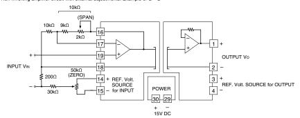
Non-inverting amplifier circuit zero/span adjustments
