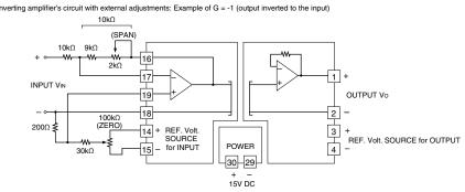
Inverting amplifier circuit zero/span adjustments
