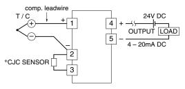
\*Deleted with B thermocouple
