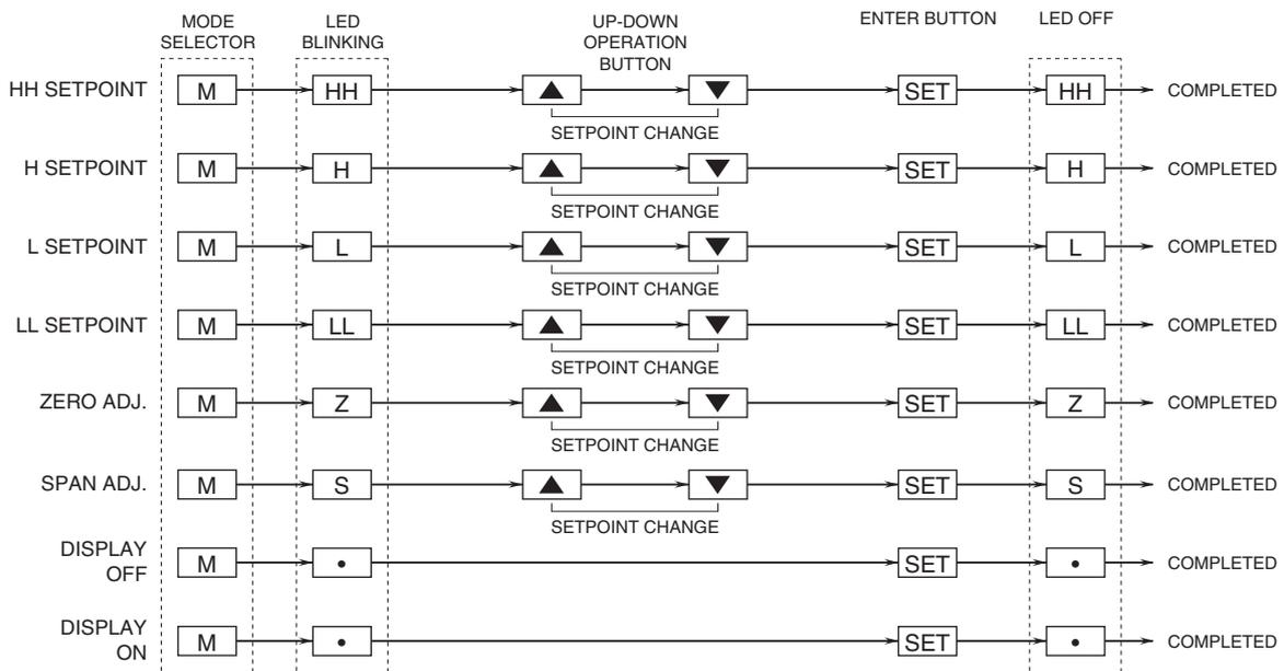
Remark 1: HH, H, L and LL setpoints are stored in the memory even the power is lost during operation.
