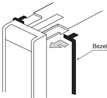
• When installing the meter into a panel, first remove the nameplates at the top and bottom of the front panel. Turn the screws behind these nameplates clockwise until the retaining clips come up and are fixed. Turning the screws counterclockwise loosen the retaining clips.
