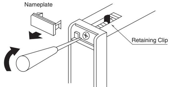
• The acrylic front cover and scaleplate can be removed when you remove the nameplates.
