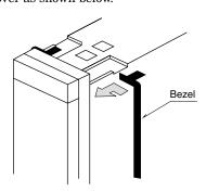
When multiple units are to be clustered side by side, insert one bezel between two units as shown below.
