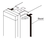
When multiple units are to be clustered side by side, insert one bezel between two units as shown below.
