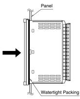
2) Push the mounting brackets into the grooves on top and bottom of the rear module, until they hit the panel's rear side.
