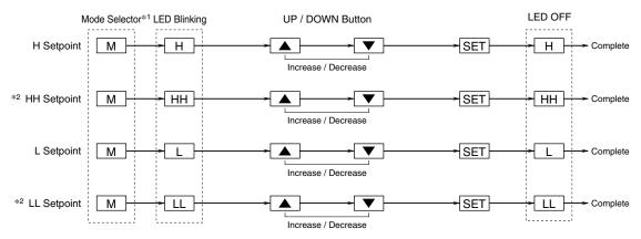
\*1. Keep pressing at least for 3 seconds to activate Mode Selector M. Press briefly for second and more times within 1 minute after it has been activated. \*2. HH or LL setpoints are not provided for the 48NAVA-2.
