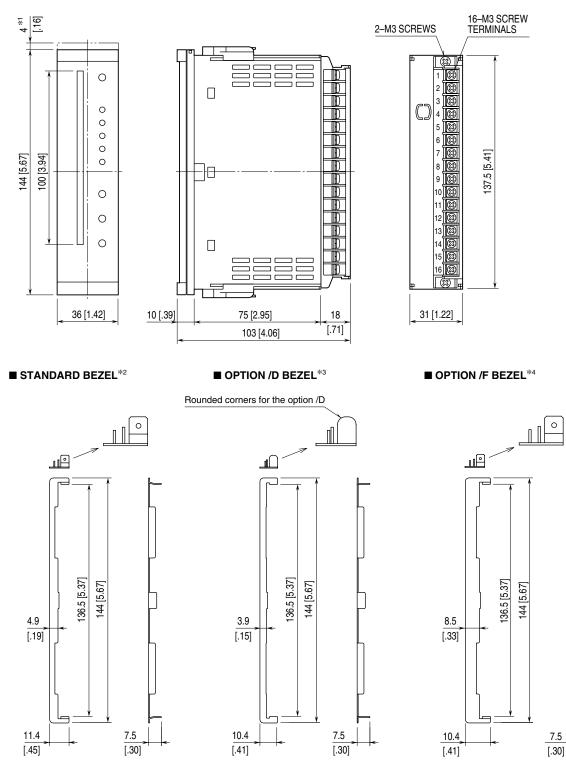
\*1. Space required when replacing the scale plate.
