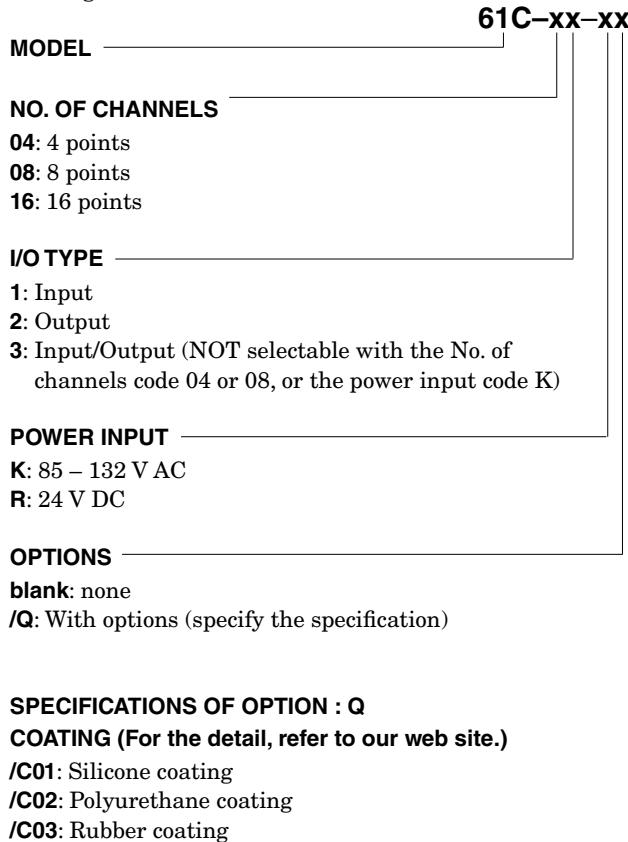
Various inputs and outputs are available by employing Mini-M series, Pico-M series or other signal conditioners. The 61C input module converts analog inputs (0 – 100%) proportionally into 16-bit signed binary signals. The one for output converts 16-bit signed binary signals proportionally into analog outputs (0 – 100%).
