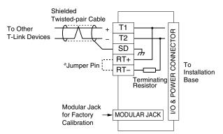
\* When the unit is located at the end of transmission line via twisted-pair cable (= no cross-wiring), short across the RT+ and RT- terminals with the jumper pin (or wire) provided with the unit.
