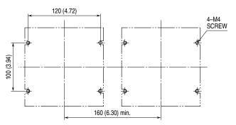
Observe at the minimum of 30 mm (1.2") for ventilation in all directions.
