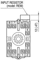
Input shunt resistor attached for current input.
