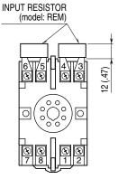
Input shunt resistor attached for current input.
