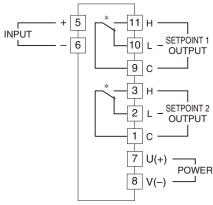
\*Relay status for output codes "1" & "4", at power OFF.
