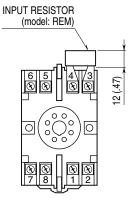
Input shunt resistor attached for current input.
