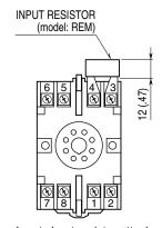
Input shunt resistor attached for current input.
