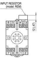
Input shunt resistor attached for current input.
