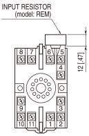
Input shunt resistor attached for current input.
