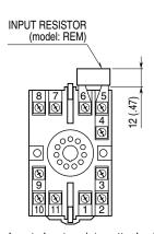
Input shunt resistor attached for current input.
