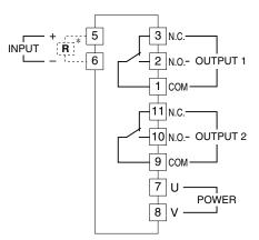
\*Input shunt resistor attached for current input.
