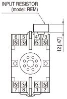
Input shunt resistor attached for current input.
