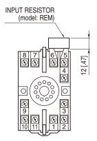
Input shunt resistor attached for current input.
