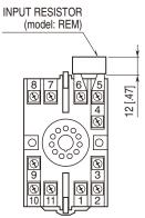
Input shunt resistor attached for current input.
