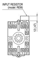
Input shunt resistor attached for current input.
