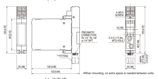
$<sup>^{\</sup>ast}$  ( ) for Rc 1/8".  $^{\ast\ast}$  Fitting provided for Rc 1/8" or 1/4" NPT connection.
