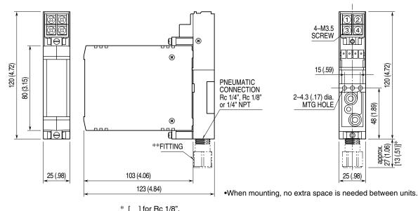
\* [ ] for Rc 1/8". \*\*Fitting provided for Rc 1/8" or 1/4" NPT connection.
