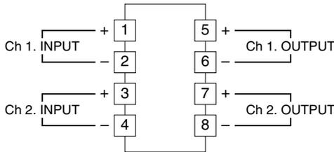
For the single-channel model, the terminals 3 – 4 and 7 – 8 are used.
