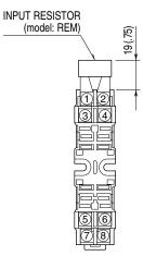
Input shunt resistor attached for current input.
