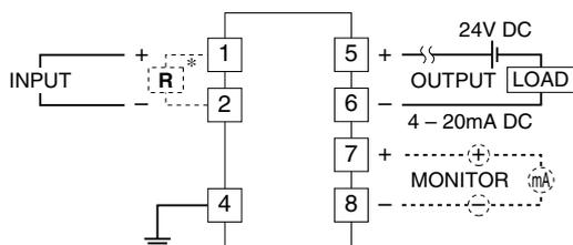
\*Input shunt resistor attached for current input.
