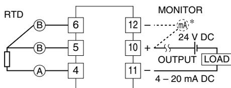
\* DC ammeter's internal resistance 10 ohms max.
