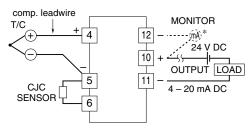
\* DC ammeter's internal resistance 10 ohms max.
