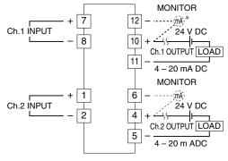
\* DC ammeter's internal resistance 10 ohms max.
