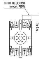
Input shunt resistor attached for current input.
