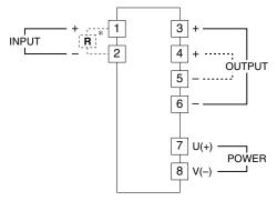
\*Input shunt resistor attached for current input.
