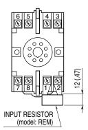
Input shunt resistor attached for current input.
