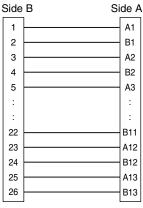
Pins No. A14 - B20 on Side A are not connected.
