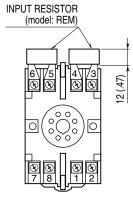
Input shunt resistor attached for current input.
