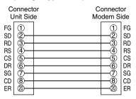
Use straight type cable as in the diagram above.
