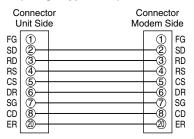
Use straight type cable as in the diagram above.
