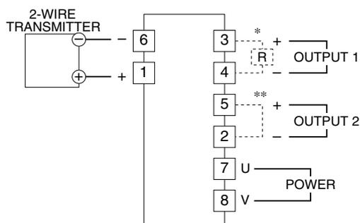
\* Use output shunt resistor for voltage output.
