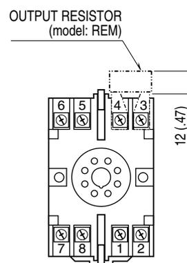
Use output shunt resistor for voltage output.
