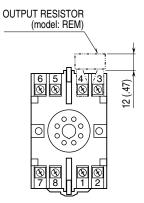
Use output shunt resistor for voltage output.
