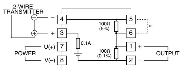
\*When the resistor [100Ω 5%] for adjusting load on the current loop is not required, short across terminals 5 – 6, or connect the 2-wire transmitter to terminals 3 (+) – 6 (-).
