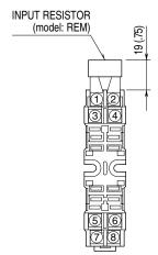
Input shunt resistor attached for current input.
