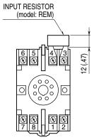
Input shunt resistor attached for current input.
