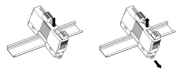
Note: When the unit is mounted on a DIN rail attached on the wall surface in vertical direction, use of an attachment plate to prevent the module from sliding down is recommended.
