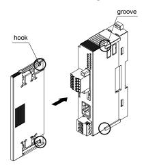
When removing the cover by DIP SW setting, pull it out while squeezing the hooks inward.
