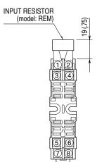
Input shunt resistor attached for current input.
