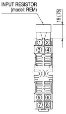
Input shunt resistor attached for current input.
