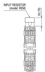
Input shunt resistor attached for current input.
