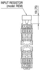
Input shunt resistor attached for current input.
