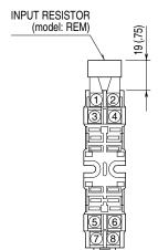
Input shunt resistor attached for current input.
