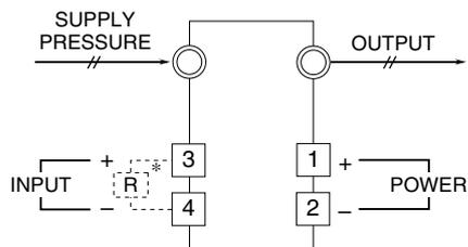
\*Input shunt resistor attached for current input.
