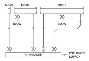
Select an appropriate pipe size for the required flow volume. Connect a stopping valve at the pipe connection to the air header for easy testing and maintenance.
