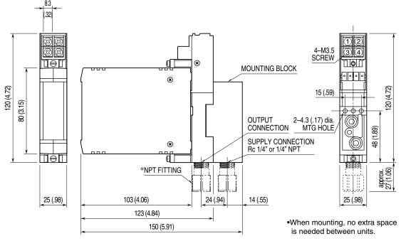
\*Fitting is provided for 1/4" NPT connection.
