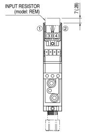
Input shunt resistor attached for current input.
